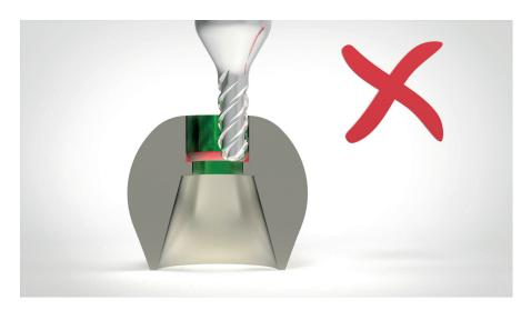
The seating for the screw head within the superstructure CANNOT be produced with the commonly used ball milling cutters.
