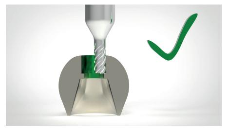
The required profile can be established only using a suitable end mill cutter (pic-ture with green checkmark).
